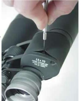
The setscrews move the image in the same direction as the screw. So when screwing the right setscrew inward (clockwise as viewed from above), the right image will move downward and also to the left. Unscrewing the right setscrew (couter-clockwise) moves the image upward and also to the right.
