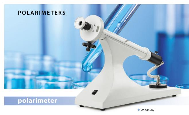
Polarimeters are suitable for fast and accurate measurements of sugars, glucose, perfume, chemical substances and medical drugs. Equipped with a Glan Thomson prism and Laurent Quartz plate, a built-in 230 V 589.3 nm sodium lamp or a high-power LED with 589.3 nm filter
