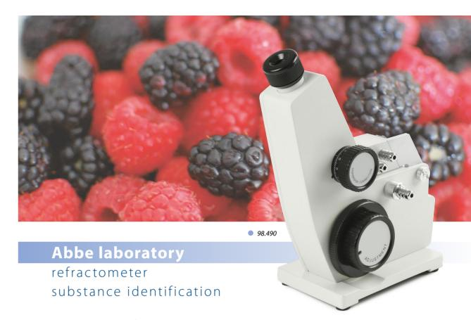
The Abbe laboratory refractometer is a bench-top instrument for high-precision measurements of an index of refraction and suitable for determination of the refractive index of solid samples, such as glass, plastics, and polymer films
