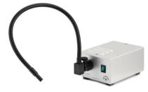
Compact cold light source with single 40 cm, 6 mm diameter fiber light conductor. Equipped with a 20 W halogen lamp. Light intensity is factory preset and can not be adjusted
