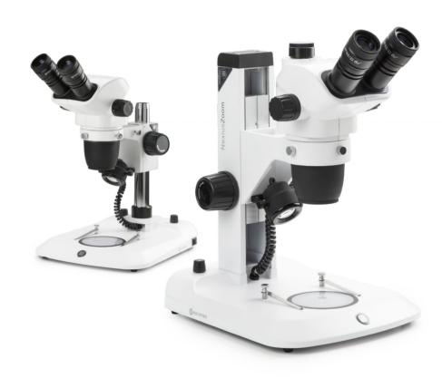
The NexiusZoom stereo microscopes of Euromex enable examining your specimen with high-performance precision and they generate two- and three -dimensional images, which make them highly suitable for your demanding microscopy applications
